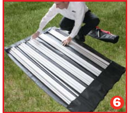
6 Unroll the Blast Pole Bag to reveal the five Blast poles and hardware. Note that each pole is connected together in the order of their installation with bungee cord. The largest diameter pole will serve as the base and the smaller diameter poles will gradually get smaller toward the top.
